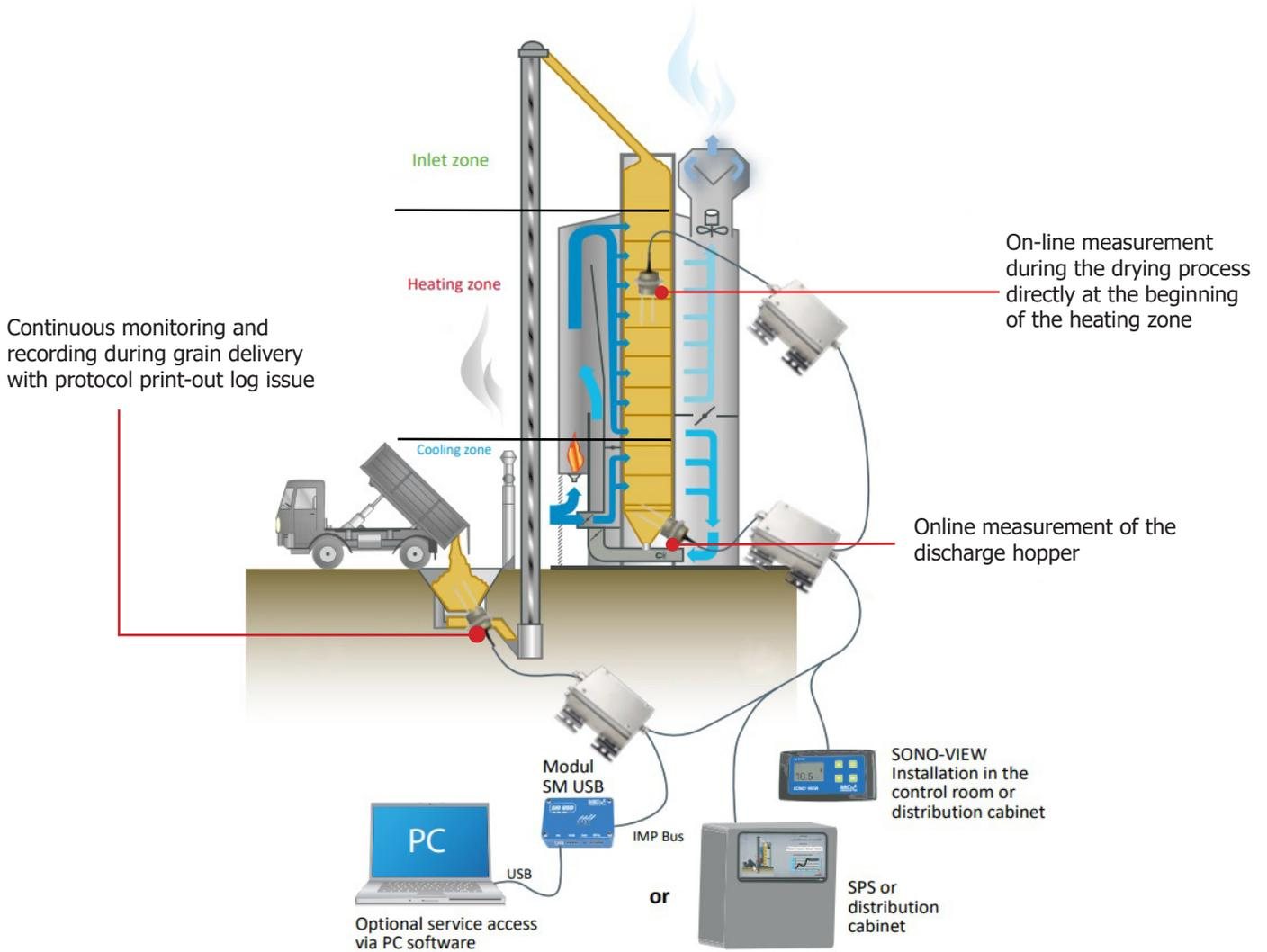
*Note : The **TRIME-EX-GWs-GR** can resist temperature up to 0...120°C (short-time up to 150°C). Thus, do not use the probe above range of temperature.*
